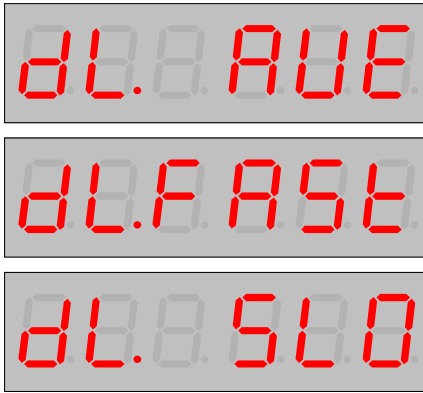
Figure 7: Reporting Data Link Speed Option. “dL.” is displayed with an “AVE”, “FAST”, or “SLO” value. Setting the On/Off Switch to “Off” sets the value to AVE, the typical speed for the Data Link (top). Changing the On/Off Switch to “Weigh” alternates the value between FAST (middle) and SLO (bottom) to slightly speed up or slow down the Data Link.
