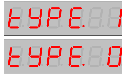
Figure 5: Typewriter Display Option. “tYPE.” is displayed with a 1 or 0 value. Setting the On/Off Switch to “Weigh” changes the value to 1 and turns on Typewriter Display option (top). Setting the switch to “Off” changes the value to 0 and turns off Typewriter Display Mode (bottom).
